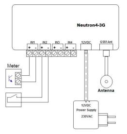
For example JAMAK 2x(2+1)x0,5mm2 instrumentation cable can be used between the meter and Neutron4-3G. The open collector or relay output of a single meter is connected to Neutron4-3G as shown above.
