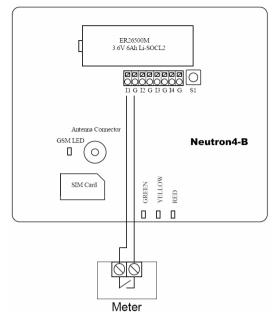
For example JAMAK 2x(2+1)x0,5mm2 instrumentation cable can be used between the meter and Neutron4-B. The relay output of a single meter is connected to Neutron4-B as shown above.
