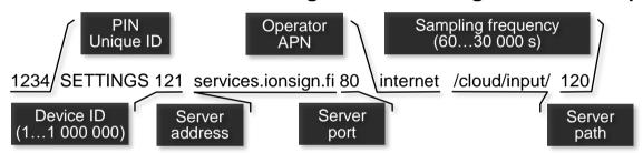
The example command sets device **121** to collect and transfer data with two-minute intervals (**120**s) to server **services.ionsign.fi**, path **/cloud/input/** and port **80**, using **internet** as APN. The device specific PIN code **1234** precedes the actual command.
