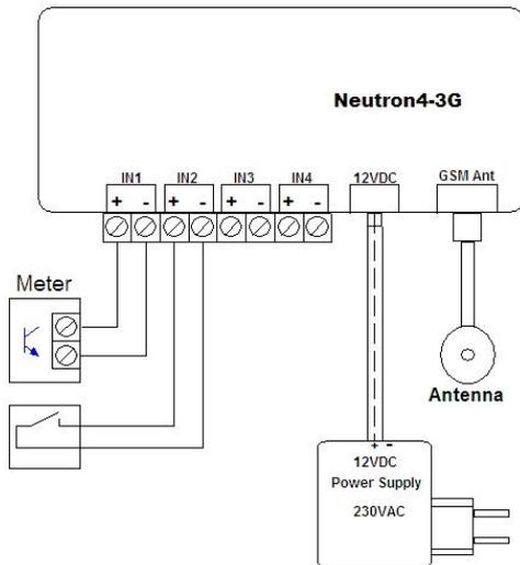
For example JAMAK 2x(2+1)x0,5mm2 instrumentation cable can be used between the meter and Neutron4-3G. The open collector or relay output of a single meter is connected to Neutron4-3G as shown above.
